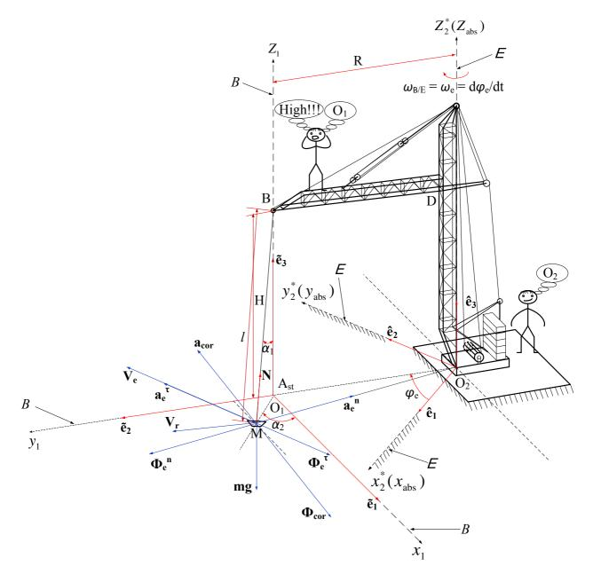
Figure 3. Computational scheme, illustrating concepts of Foucault pendulum-like systems in mechanical engineering problems of boom crane dynamics and control
