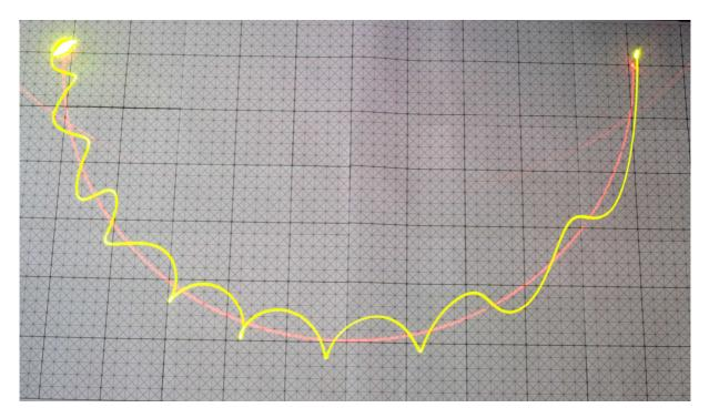
Figure 1. Educational physical simulation-based experiment, illustrating influence of Coriolis effects on the shape of an absolute LED's yellow zig-zag-shaped trajectory
